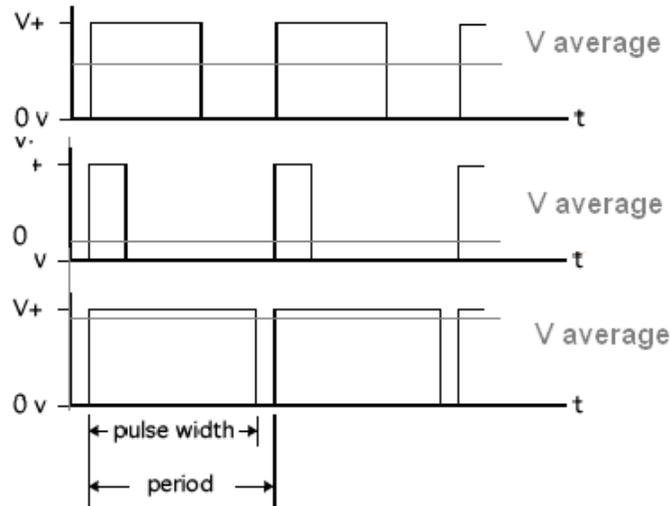
**Illustration of Pulse Width Modulation (PWM)**
