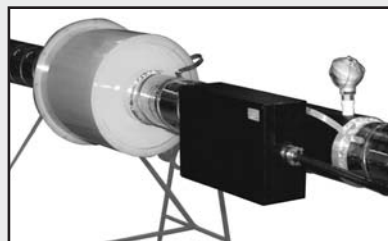
Impedance Heating System
